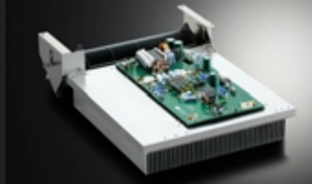
PA unit and heat sink
